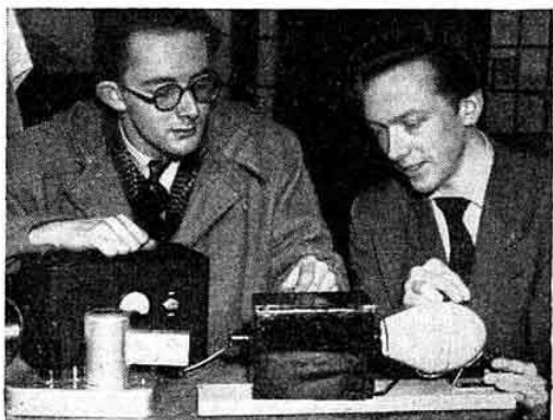
P. Gowen, G3IOR (left) and D. C. Money, G3HKD, with the light beam apparatus they built for the Amateur Radio and Model Aircraft Exhibition held in Norwich from April 6 to 10. The light transmitter on the right is modulated by pieces of polarised glass operated from telephone ear pieces.
